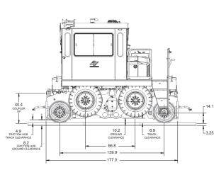
**Frame Heavy-duty one piece, welded from 2" steel plate.** Full width bumpers incorporate powertrain protection into design.
