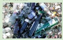
The glass is crushed into small pieces, which are fed into a burner that heats and tumbles the glass until all the labels and other unwanted materials burn off, leaving clean, tumbled glass pieces.
